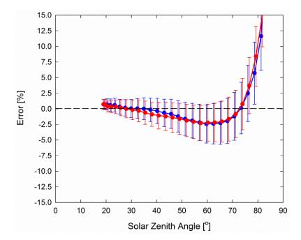
Mean cosine response of twentythree SQ series quantum sensors (error bars represent two standard deviations above and below mean). Cosine response measurements were made by direct side-by-side comparison to the mean of four reference thermopile pyranometers, with solar zenith angle-dependent factors applied to convert total shortwave radiation to PPFD. Blue points represent the AM response and red points represent the PM response.
