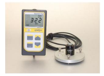
The AL-100 leveling plate is recommended for use with the MQ-200. To facilitate mounting to a cross arm, the AM-110 mounting bracket is recommended for use with the AL-100.
