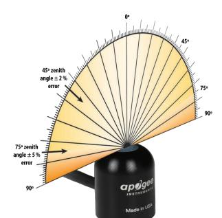
Directional, or cosine, response is defined as the measurement error at a specific angle of radiation incidence. Error for Apogee SQ series quantum sensors is approximately  $\pm 2$  % and  $\pm 5$  % at solar zenith angles of 45° and 75°, respectively.
