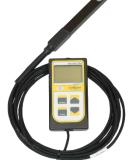
MQ-300 Series: Meter w/ separate line sensor
