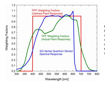
Radiation weighting factors for PPFD (defined plant response to radiation), YPFD (measured plant response to radiation), and Apogee quantum sensors (sensor sensitivity to different wavelengths of radiation).
